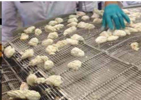
GEA MultiDrum breading process
